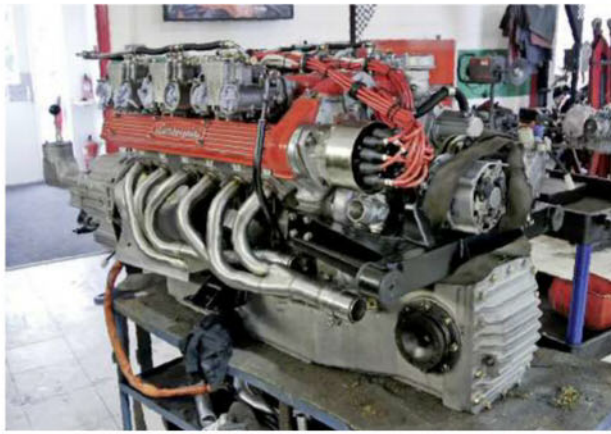
Just setting the valve clearances of the Lamborghini V12 was a two-day job
