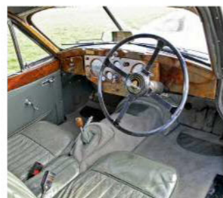
Good headlining, carpets and dashboard timber, but the seats are torn in places
