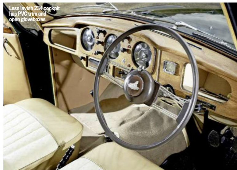
Riley has adjustable steering column but right-hand gearchange
