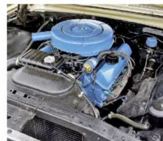
6.4-litre V8 has a recored radiator, rebuilt carburettor and new exhaust manifolds
