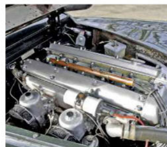
XK engine has twin SU HD8 carburetors, original radiator and mesh air filters
