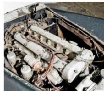
1952 XK engine has replaced the old Alvis straight-six previously fitted to go racing
