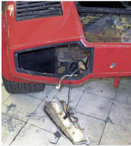
Lights were bonded in and all the glue had to be picked out
