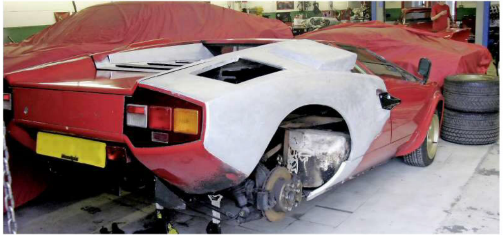
New rear wing was hand-beaten out of an aluminium sheet. An unused right-hand rear wheelarch extension was found on eBay in the US
